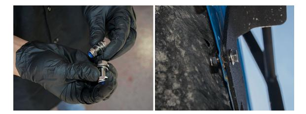
With all bolts started, move back to the top two 5mm allen bolts and finish tightening them up. You will need to push down on the Roof Rack to lock it into place.
