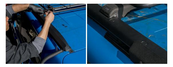
Now that everything is secure at the in the top portion of the installation, finish tightening the bottom two 13mm bolts.
