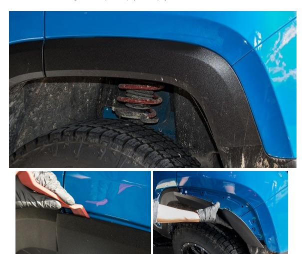
You may break some of the existing fender clips while removing the Fender Cover. The Jeep Renegade Roof Rack Ladder includes replacement clips for the re-installation.
