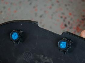
You will also need to cut two of the Fender Clip Mounts off of the back of the Fender Cover.
