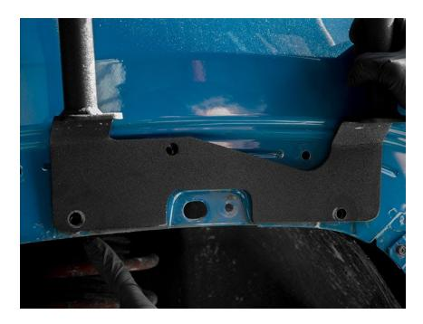
Insert the included 13mm bolts onto the mounting holes. Once you have the bolts all the way through, add the included washer and nut. Begin to tighten the two 13mm nuts.
