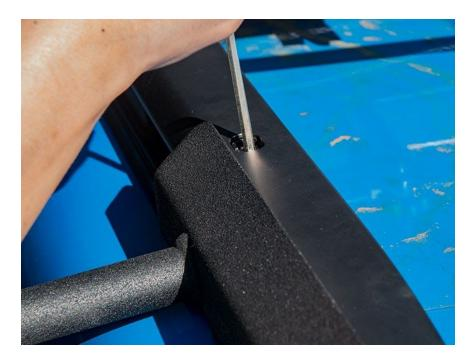
Align the bottom two holes on the Roof Rack Ladder with the two mounting holes on the Jeep Renegade Fender.
