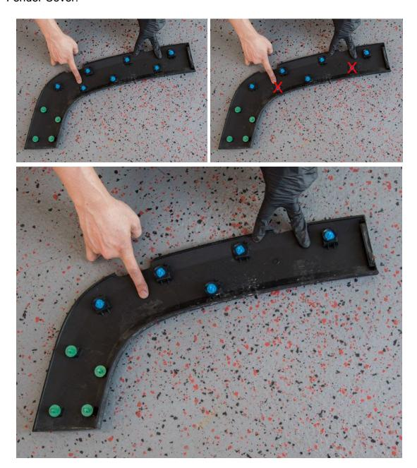
Once the Fender Cover fits properly, install the new clips that are included with the Roof Rack Ladder Kit. Push the clips back into the rear fender.
