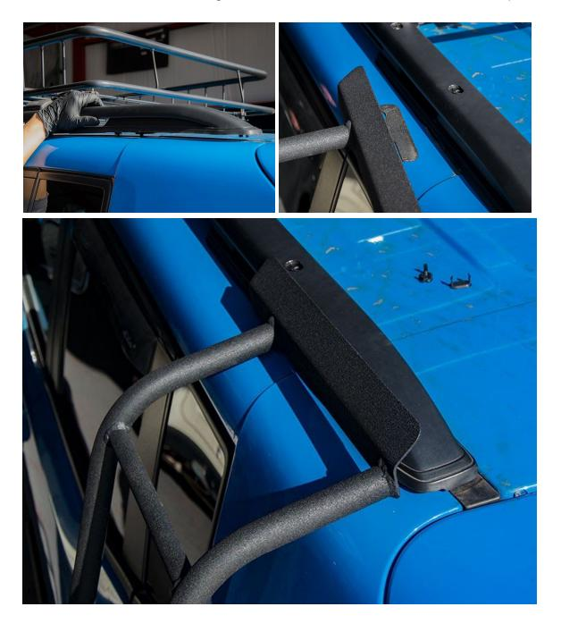
Begin to tighten the 5mm allen bolts. Leave the bolts loose enough to be able to align the bottom of the Roof Rack Ladder with the bottom mounting holes.
