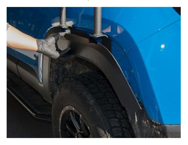
Please note: Do not insert the Fender Clips into the fender until the cover is completely trimmed and fitting properly as you may risk getting the fender clips stuck into the fender.
